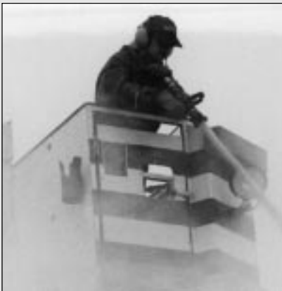
Hot water under pressure in a tight stream was required to break ice free from an aircraft wing.
